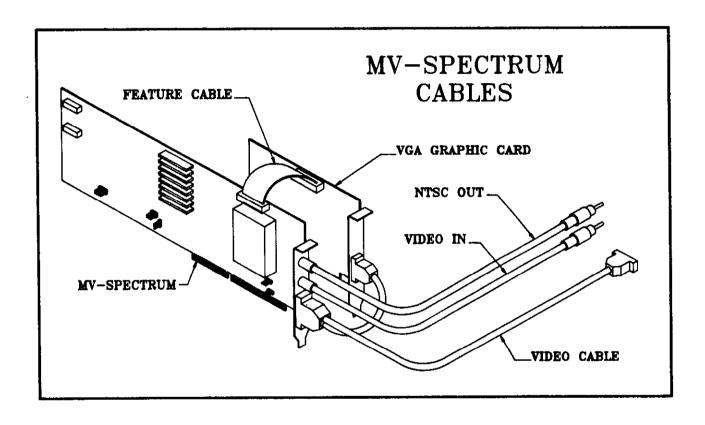
Figure 5 Connecting the Cables.
